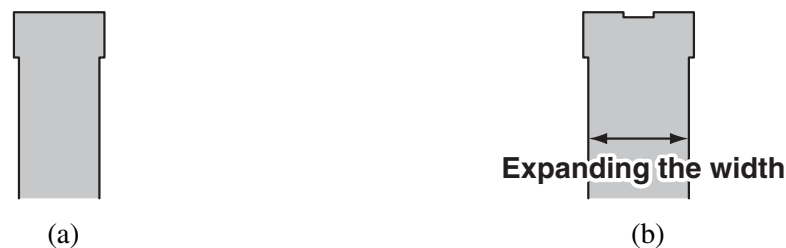
Figure 6.10 The change of the OPC pattern from (a) hammer head style to (b) serif style.
