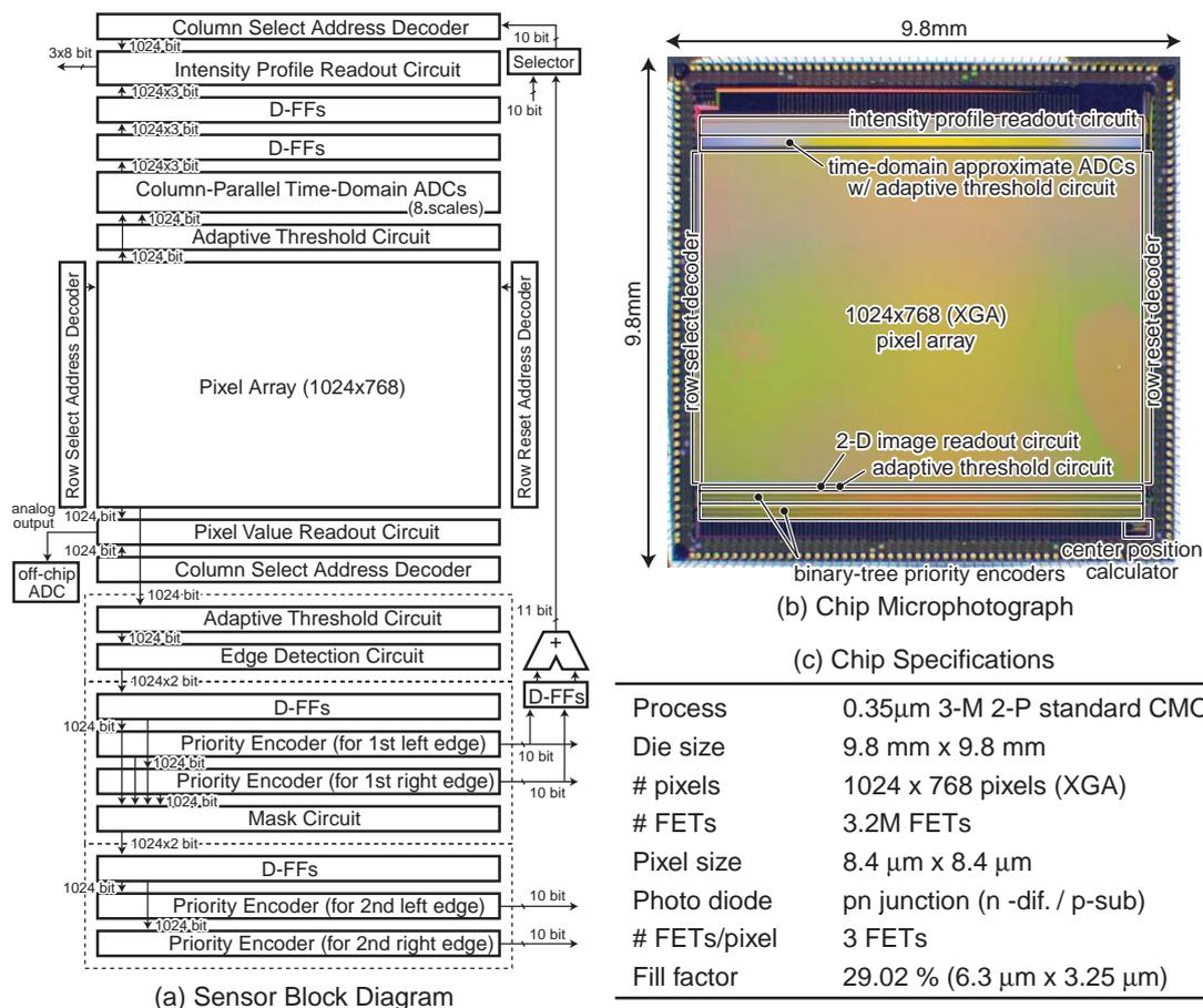
Figure 5: XGA 3-D image sensor: (a) block diagram, (b) microphotograph (c) specifications.
