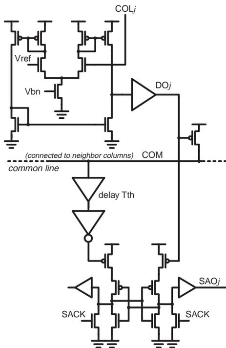
Figure 3: Schematic of adaptive threshold circuit in column.
