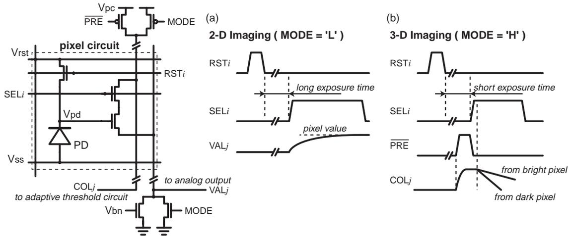
Figure 2: Pixel circuit configuration and operation: (a) 2-D imaging, (b) 3-D imaging.
