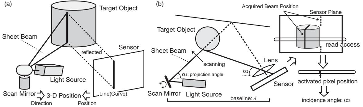
Figure 1: Light-section 3-D measurement system: (a) birds-eye view, (b) top view.
