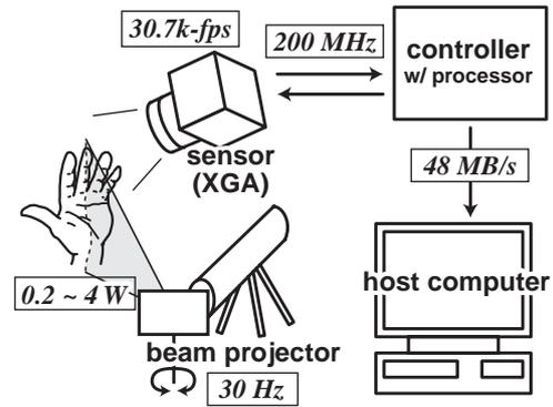
Figure 10: System requirements of real-time range finding.
