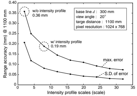
Figure 7: Possible range accuracy of XGA 3-D image sensor.
