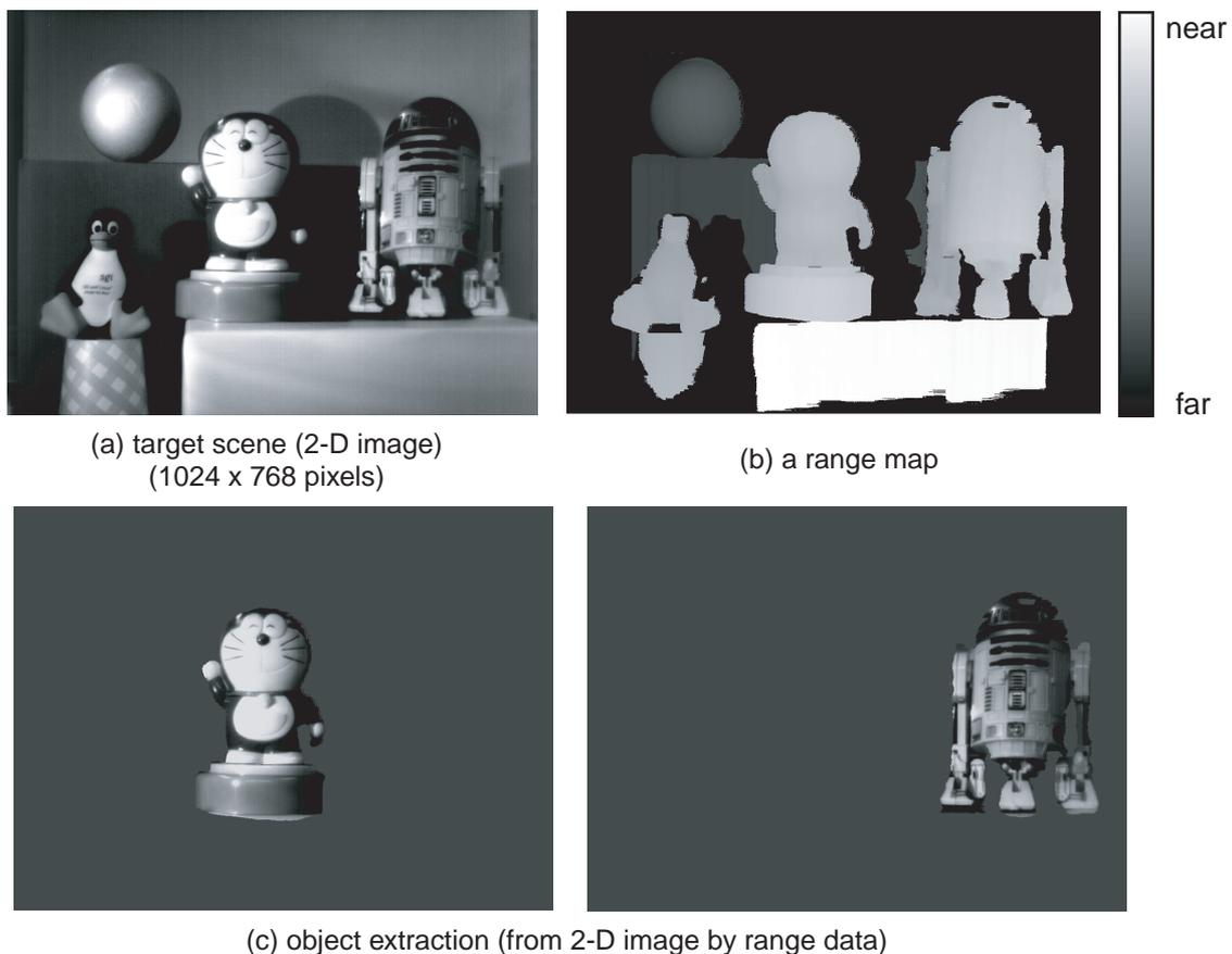
Figure 8: Measured images and object extraction: (a) a 2-D image with 1024  $\times$  768 pixels, (b) a range map, (c) object extraction using range information.
