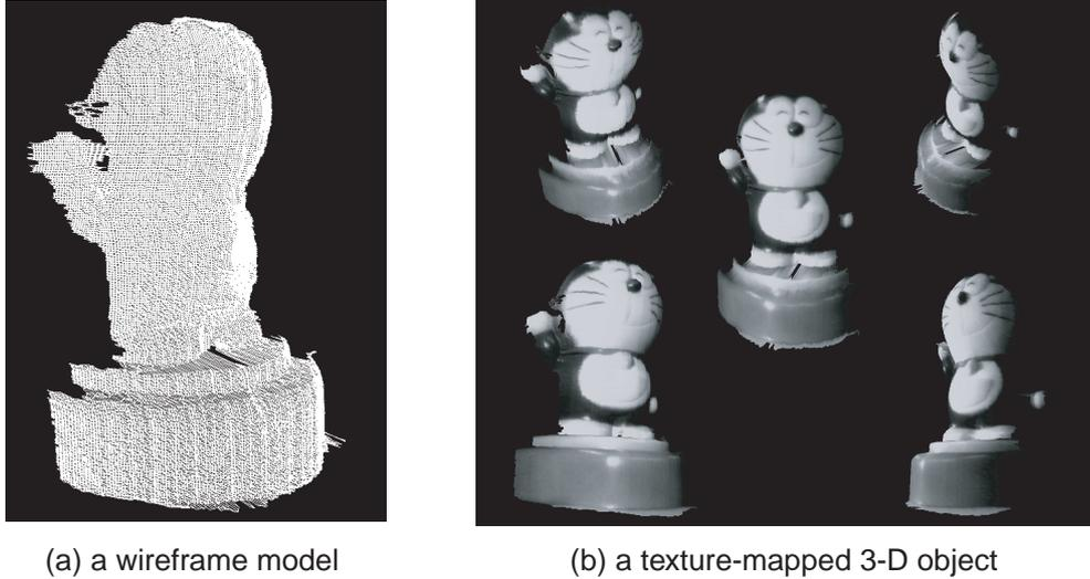
Figure 9: Reconstructed 3-D images: (a) a wireframe model, (b) a texture-mapped 3-D object.
