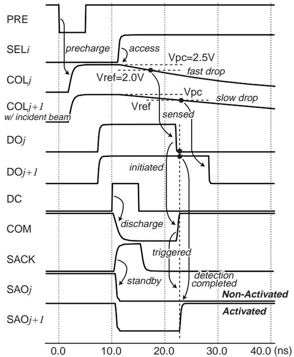
Figure 4: Simulation waveforms of activated pixel detection using 0.35  $\mu\text{m}$  CMOS process.
